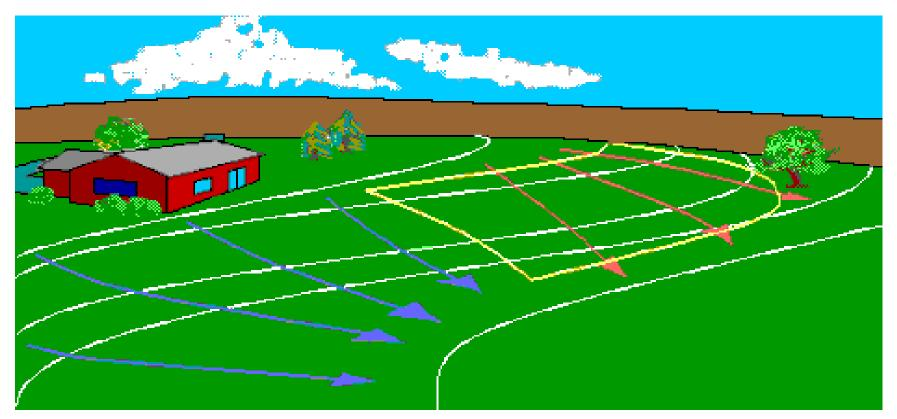
The best location for an absorption field on the site is where flow will diverge (note the red flow lines). Areas where water naturally converges (note blue flow lines) should be avoided.
