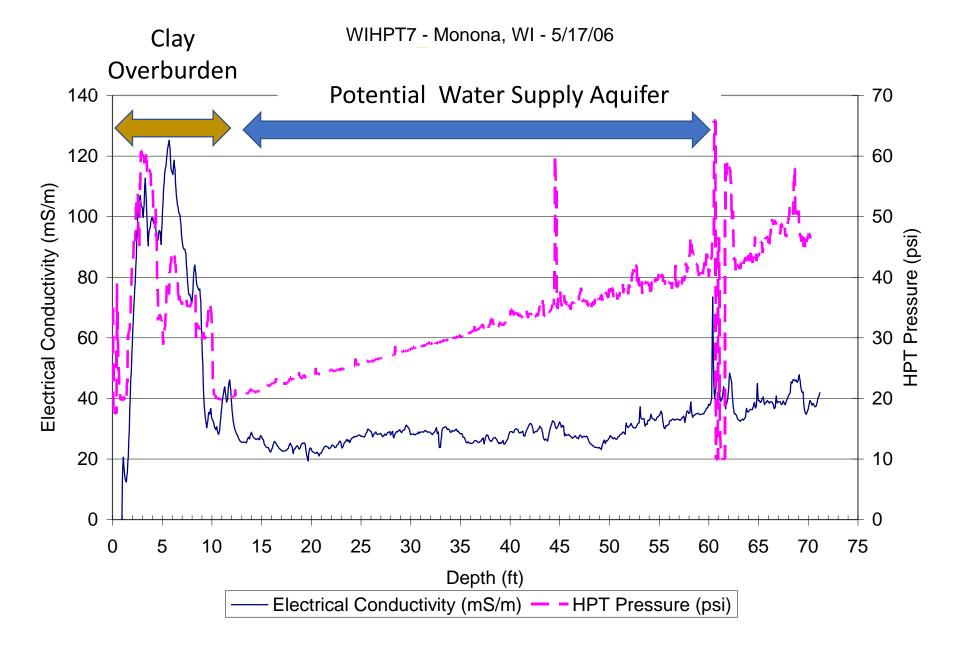
Use the geophysical and site characterization tools to install monitoring wells that sample the aquifer in the same way a water production well would sample the aquifer. (Screen across the aquifer. Do something better than a five foot screen set across the water table).
