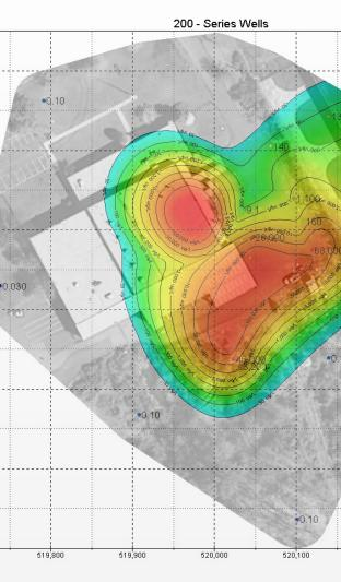
Post-Remediation 1.1.1-trichloroethane Concentrations in Overburden Groundwater (100-Series Wells) and Bedrock Groundwater (200-Series Wells)
