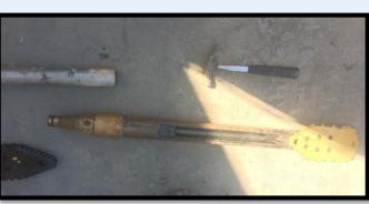
Drill bit housing with sonde
