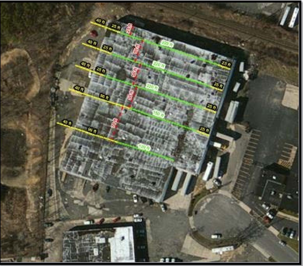
Horizontal Sub-Slab SVE well layout
