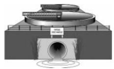
A sanitary sewer overflow occurs when there is a release of sewage from a collection system, including pipes, before it reaches a municipal wastewater treatment plant. Sewer overflows are a chronic and growing problem. Many of the nation's urban sewage collection systems are aging. Some sewers are 100 years old. Many systems have not received the necessary maintenance and repair that keeps them functioning properly.
